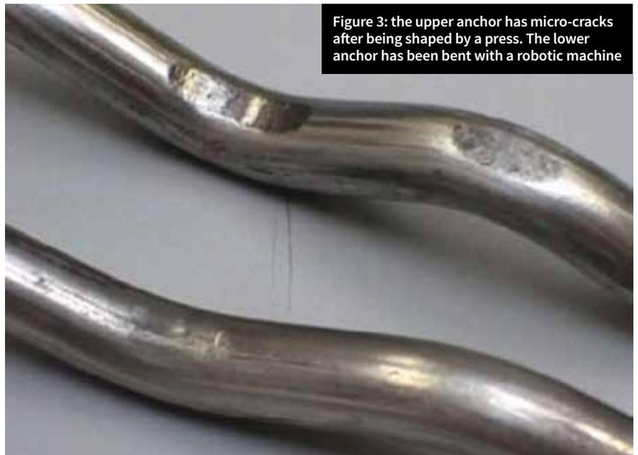
Figure 3: the upper anchor has micro-cracks after being shaped by a press. The lower anchor has been bent with a robotic machine
