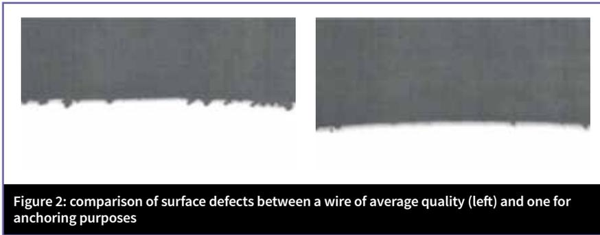
Figure 2: comparison of surface defects between a wire of average quality (left) and one for anchoring purposes
